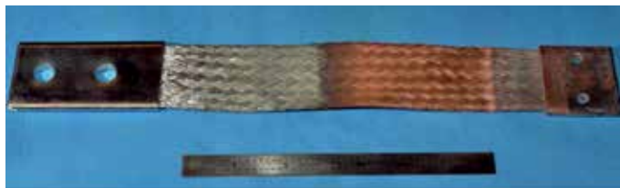
Tinned and bare copper cable sample prior to exposure
