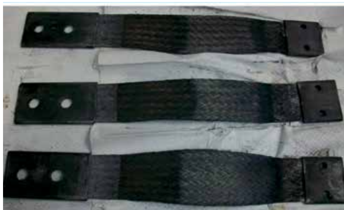
The aluminum cable samples are in nearly identical condition before and after 14 days of immersion in the H 2 S saturated test solution, see below
