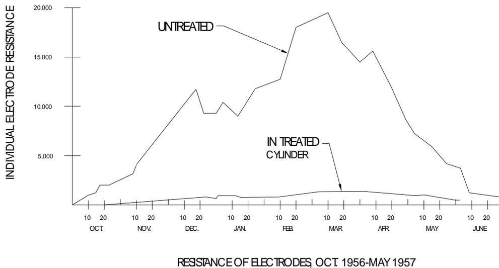
Figure 10: Ground Rods in Permafrost, Army Corps of Engineers, Point Barrow, Alaska
