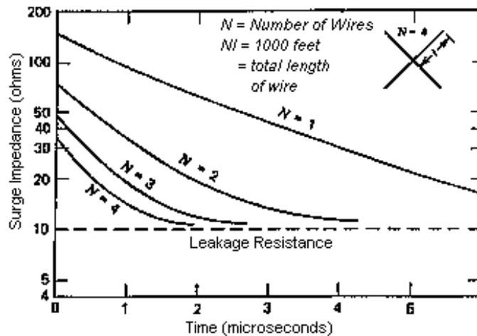
Figure 11: Surge Impedances of Various Wire Lengths
