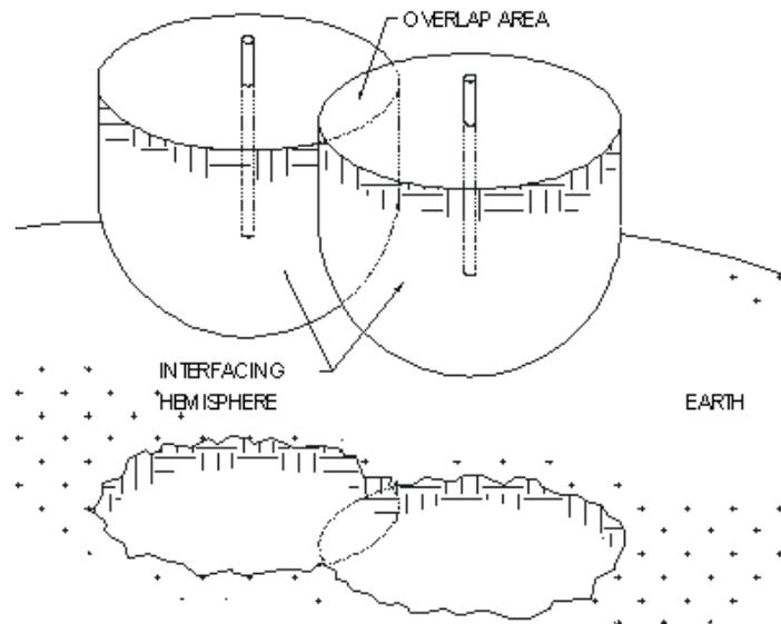
Figure 6: Overlapping Interfacing Hemispheres from Ground Rods Spaced Too Closely
