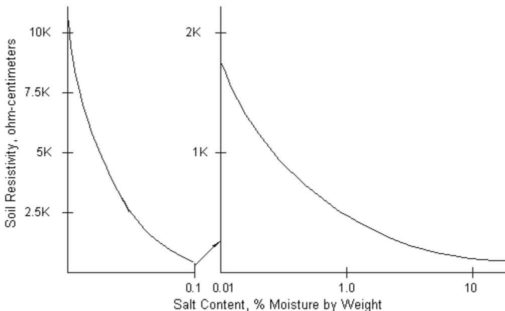
Figure 8: The Influence of Salt on Soil Resistance
