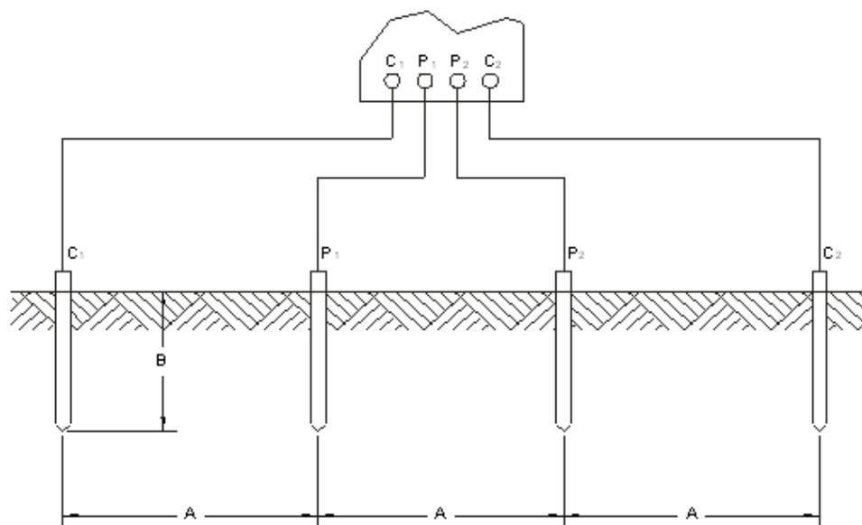
Figure 1: Soil Resistivity Testing Using Four Point Method
