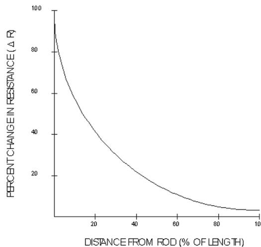
Figure 4: Measured Resistance Change as a Function of Distance from the Ground Rod
