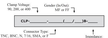
BNC or F-Type Connector = 75  $\Omega$ BNC, TNC, N, 7/16 or SMA =  $50 \Omega$
