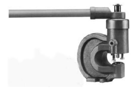
This heavy duty portable Punch Assembly is ideal for punching requirements, where holes cannot be created by conventional drilling procedures. The RGA Punch Assembly has a rated capacity of 20 tons and will punch 7/16 inch\* diameter holes in mild steel up to 1/2 inch thick. It can be used to punch holes in flat sheets and angles.
