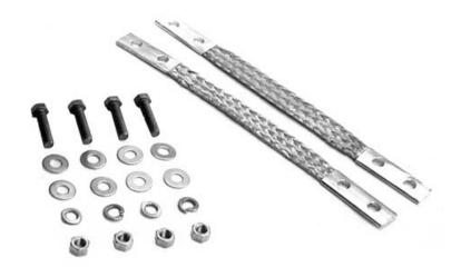
One pair of End Straps is required to attach the main conductor of each RGA to the floating roof of the tank. The RGA conductor is typically attached to the foam dam. Each RGA comes with a pair of End Straps and Hardware as part of the original equipment. These are replacements in case the original End Straps tear or break.
